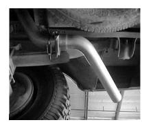
5. Slide turn out pipe # D on the tailpipe behind the rear tire. Roll turnout pipe until you have it at the correct angle for your truck and clamp # H. Spare tire may need to be loosened and pushed to the rear to allow for clearance.
