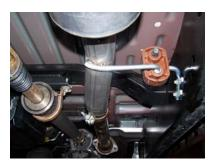
INSTALL HEADPIPE # A INTO STOCK PIPE. THE END OF THE PIPE SHOULD BE AT THE 12 O'CLOCK POSITION,. INSERT WELDED HANGERS INTO RUBBER GROMMET. ATTACH WITH FACTORY CLAMP. DO NOT TIGHTEN.
