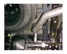
**INSTALL OVERAXLE** TAILPIPE #C INTO MUFFLER 1  $\frac{1}{2}$ " TO 2". **INSERT HANGERS INTO** RUBBER GROMMETS.USE CLAMP #E TO SECURE PIPE TO MUFFLER.DO NOT TIGHTEN.
