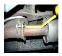
TO REMOVE YOUR STOCK EXHAUST, MEASURE 6" FROM THE 2-BOLT FLANGE LOCATED IN FRONT OF YOUR STOCK MUFFLER AND CUT.
