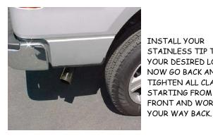
MAKE SURE YOU HAVE A 1" CLEARANCE ON ALL RUBBER BRAKE LINES, SHOCK BOOTS, TIRES, FUEL LINES, ETC..
