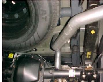
INSTALL OVERAXLE TAILPIPE #C INTO MUFFLER 1 1/2" TO 2". INSERT HANGERS INTO RUBBER GROMMETS. USE CLAMP #E TO SECURE PIPE TO MUFFLER. DO NOT TIGHTEN.
