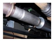
2. To remove your stock exhaust, remove the clamp located just behind the converter. Disengage the welded hangers from the OEM rubber grommets. Use WD-40 to aid in the process. Do not damage or remove the rubber grommets as you will re-use them. Now, cut off tailpipe and remove exhaust.
