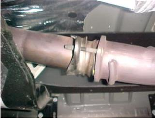
**1.** To remove the stock exhaust, remove it from the clamp located just behind the catalytic converter. Disengage the welded hangers using WD-40 from the OEM rubber grommets. Do not damage or remove the rubber grommets as you will re-use them to mount your new system. Now, un-bolt and remove the catalytic converter from the 2-bolt flange.
