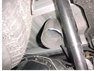
**5.** Install the over axle tailpipe #C into the muffler 1½-2" and secure with clamp #G. DO NOT TIGHTEN.
