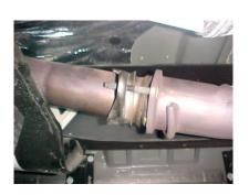
TO INSTALL YOUR GIBSON DOWN PIPE YOU NEED TO REMOVE YOUR STOCK EXHAUST. REMOVE THE STOCK EXHAUST FROM THE CLAMP LOCATED JUST BEHIND THE CATALYTIC CONVERTER. CUT OFF YOUR STOCK TAILPIPE FOR EASIER REMOVAL. LEAVE ALL RUBBER GROMMETS IN PLACE. USE WD-40 TO AID IN REMOVAL OF EXHAUST AND HANGER. AFTER YOUR STOCK EXHAUST IS REMOVED YOU NEED TO REMOVE THE CATALYTIC **CONVERTER FROM THE 2-**BOLT FLANGE.
