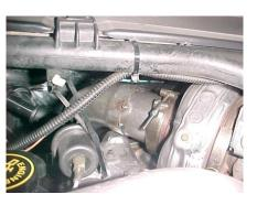
REMOVE THE REMAINING STOCK DOWN PIPE BY UNCLAMPING IT FROM THE TURBO HOUSING. USE A 11MM SOCKET OR WRENCH. REMOVE YOUR STOCK PIPE THROUGH THE BOTTOM. DO NOT DISGARD THE STOCK CLAMP YOU WILL NEED TO RE-USE IT.
