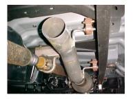
Install head pipe # A on to your existing stock front pipe and line up the notch. Then secure with clamp # H. Insert hangers into rubber grommets. Do not tighten.
