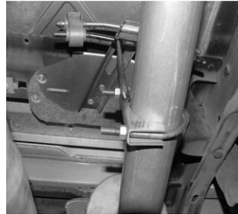
INSTALL OVERAXLE TAILPIPE #C INTO THE MUFFLER NO MORE THAN 1 1/2" TO 2". INSERT WELDED HANGER INTO RUBBER GROMMET. USE CLAMP #G TO ATTACH T-HANGER # H ONTO OVERAXLE TAILPIPE AND INSERT INTO RUBBER GROMMET. THE HANGER SHOULD BE FACING TOWARDS THE DRIVERSIDE. MAKE SURE YOU HAVE EQUAL SPACE BETWEEN SHOCK AND SPARE TIRE. THE SPARE TIRE MAY NEED TO BE LOOSENED AND PUSH TO THE DRIVER SIDE AND THEN ROTATE TO GAIN CLEARANCE. FX4 MODELS MAY NEED TO REMOVE RIGHT REAR SHOCK BOOT
