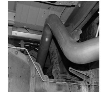
INSTALL TURNOUT PIPE #D TO THE OVERAXLE TAILPIPE. ROTATE PIPE SO IT IS AT THE CORRECT ANGLE FOR YOUR VEHICLE. USE CLAMP #G TO ATTACH.
