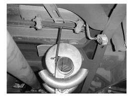
MAKE SURE YOU HAVE A MINIMUM OF 1" CLEARANCE ON ALL PIPES RUBBER BRAKE LINES, SHOCK BOOTS, TIRES, ETC...
