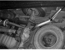
Slip tailpipe #C into muffler no less than 1-1/2" and no more than 2" and attach with hanger # H and clamp # G to connect 10" hanger to rear of tailpipe. DO NOT TIGHTEN
