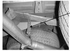
Install rear tailpipe hanger #I. Measure from rear of frame 21" forward to slotted hole. Place bolt with large washer from inside frame out. Put 10" hanger on outside of frame. Bolt through top hole, put lock washer and nut on and tighten. End of hanger swivels so it can be adjusted for 3" clamp.
