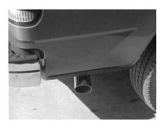
Slip stainless steel tip on and clamp down. To clean stainless tip use any stainless steel or aluminum cleaner. Firmly tighten all bolts and clamp down securely.
