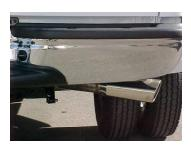
Install the over axle tailpipe # C into the muffler 1-1/2" to 2". Secure to the muffler using clamp # H Do not tighten. You may need to loosen spare tire & push over towards driverside & re tighten. Next install exit pipe # D onto overaxle pipe insert hanger into rubber grommet. Use clamp # H to secure pipes together rotate to proper angle for your vehicle. DO NOT TIGHTEN.
