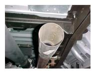
Install head pipe # A on to your existing stock front pipe and secure with clamp # I. Do not tighten.
