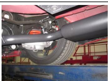
3. Now install the passenger side tailpipe assembly #B by sliding the metal hangers into the rubber grommets. Use clamp #D to secure together.
