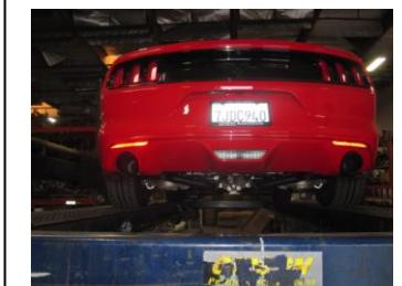
5. When you have everything in Place, firmly tighten all bolts And clamps down securely Use stainless steel cleaner and weekly to prevent tip from discoloration. Inspect all fasteners after 25-50 miles of operation and re-Tighten as necessary
