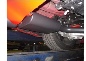
4. Now do the same procedure for the driver side. Use clamp # D to secure to the muffler.
