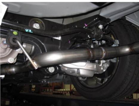
5. Now do the same procedure for the driver side. Use clamp # D to secure to the muffler. When you have everything in Place, firmly tighten all bolts And clamps down securely. Be sure you keep an eye on the tip position as it can move during the tightening process,
