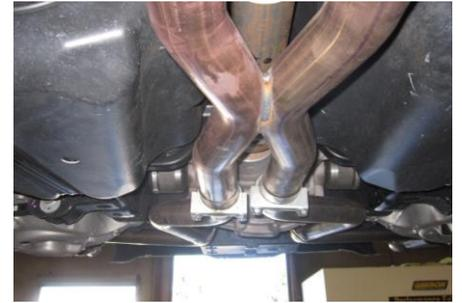
4. Now install the passenger side tailpipe assembly #B by sliding the metal hangers into the rubber grommets. Then do the same for the driver side muffler assembly #A. Use clamp #D to secure together
