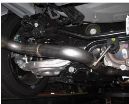
6. Use stainless steel cleaner to prevent tip from discoloration. Inspect all fasteners after 25-50 miles of operation and re-Tighten as necessary
