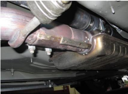
2. Install your Gibson muffler assembly using the stock clamps do not tighten.
