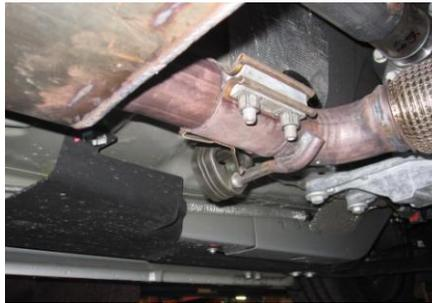
3. With the muffler assembly in place be sure the muffler sits level and is supported with a jack stand.
