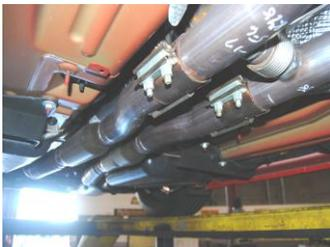
2. Loosen up the 2 clamps in the middle of the vehicle and slide them over the tailpipes. Now separate both tailpipes from mufflers and slide them out. Next remove the stock mufflers by sliding them out of the stock rubber grommets.
