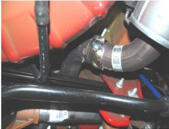
1. To remove your stock exhaust, unbolt the clamps by 15mm wrench or socket.
