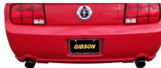
7. When you have everything in place, firmly tighten all bolts and clamps down securely. Use stainless steel cleaner and a Scotch Brite pad weekly to prevent tip from discoloration. Inspect all fasteners after 25-50 miles of operation and re-tighten as necessary.
