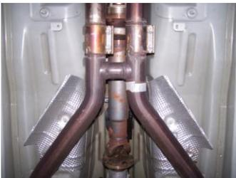
3. Loosen up the 2 clamps in the middle of the vehicle and slide them over the tailpipes. Now separate both tailpipes from mufflers and slide them out. Next remove the stock mufflers by sliding them out of the stock rubber grommets.
