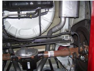
5. Install the passenger side tailpipe into muffler assembly using clamp #C to secure. Do not tighten. Use the stock clamp to secure the tailpipe to the stock h-pipe.
