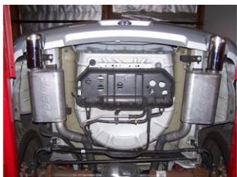
4. Now install the passenger side muffler assembly #B by sliding the metal hangers into the rubber grommets. Then do the same for the driver side muffler assembly #A.
