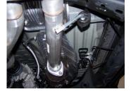
4. Install muffler onto headpipes 1.5"-2". Use a jack stand to support the muffler. Use clamps #G to secure the muffler to the headpipes. Do not tighten.
