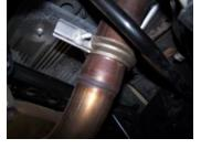
3. Install passenger side headpipe #A using your stock bolts. Do not tighten. Next, install driver side headpipe #B using stock bolts. Do not
