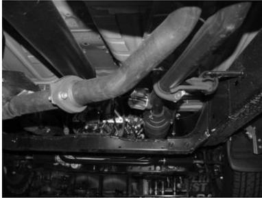
TO REMOVE STOCK EXHAUST UNBOLT THE CLAMP LOCATED BEHIND THE MUFFLER. THE TAILPIPE SHOULD SLIDE OFF. UNBOLT THE STOCK MUFFLER AND HEADPIPES FROM THE 2 FLANGES JUST BEFORE THE MUFFLER. DO NOT DISGARD STOCK NUTS AND BOLTS. LEAVE ALL RUBBER GROMMETS ON THE HANGER. USE WD-40 TO AID IN REMOVAL OF THE EXHAUST AND HANGERS.
