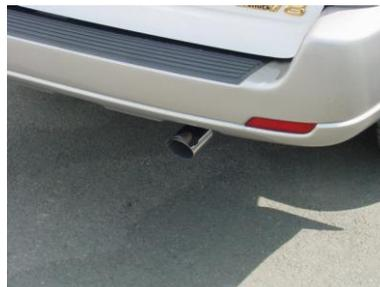
INSTALL THE STAINLESS TIP #E. TO CLEAN TIP USE ANY STAINLESS OR ALUMINUM CLEANER AND A SCOTCH BRITE PAD. NOW GO BACK AND TIGHTEN ALL NUTS, BOLTS AND CLAMPS STARTING FROM THE FRONT AND WORKING BACK.
