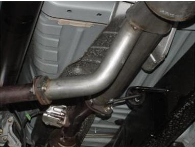
INSTALL HEADPIPE ASSEMBLY #A ONTO STOCK FLANGES, RE-USING STOCK NUTS AND BOLTS. DO NOT TIGHTEN. INSERT WELDED HANGER INTO RUBBER GROMMET.
