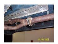
LAY OUT THE EXHAUST ON THE FLOOR SO IT LOOKS LIKE THE DRAWING AND COMPARE PARTS WITH MANUAL. TO REMOVE THE STOCK EXHAUST REMOVE IT FROM THE 2-BOLT FLANGE LOCATED IN THE FRONT OF THE MUFFLER. LEAVE ALL RUBBER GROMMETS IN PLACE. USE WD-40 TO AID IN REMOVAL OF EXHAUST AND
