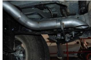
**5.** Next, install the exit pipe #D. onto overaxle pipe. Use clamp #E to secure to the tailpipes. DO NOT TIGHTEN. Insert welded hanger into rubber grommet.
