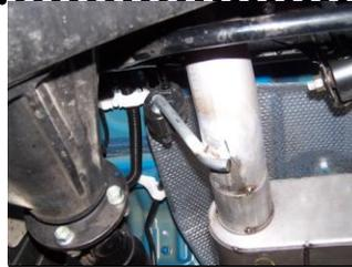
**4.** Install the overaxle tailpipe #C into the muffler 1 1/2"-2" secure with clamp #E. DO NOT TIGHTEN. Insert welded hanger into rubber grommet.
