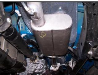
**3.** Install muffler #B onto head pipe 1 1/2"-2" with the louvers facing towards the converter. Use a jack stand to support the muffler. Use clamp #E to secure the muffler to the headpipe. DO NOT TIGHTEN.
