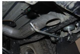
**6.** Check for all proper clearance and begin to tighten all clamps starting from the front of the vehicle. Before starting the engine be sure there is a 1" clearance from all exhaust parts.
