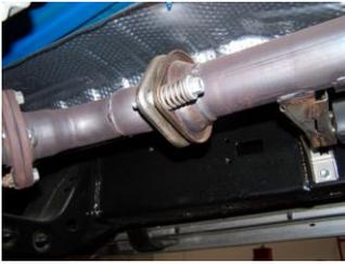
**1.** To remove the stock exhaust remove it from the 2-bolt flange located in front of the stock muffler. Disengage the welded hangers using WD-40 from the OEM rubber grommets. Do not damage or remove the rubber grommets as you will re-use them to mount your new system. Now, cut off tailpipe and remove exhaust.
