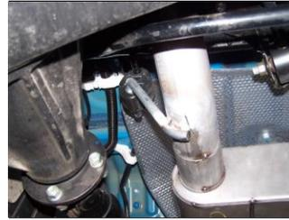
**4.** Install the overaxle tailpipe #C into the muffer 1½-2" secure with clamp #F. DO NOT TIGHTEN. Insert welded hanger into rubber grommet.
