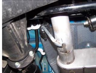
**4.** Install the overaxle tailpipe #C into the muffer 1½-2" secure with clamp #F. DO NOT TIGHTEN. Insert welded hanger into rubber grommet.
