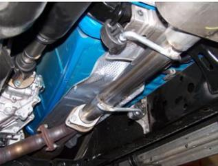
**2.** Install head pipe #A onto your existing stock front pipe and attach with hardware kit #G. DO NOT TIGHTEN. Insert welded hangers into rubber grommets.
