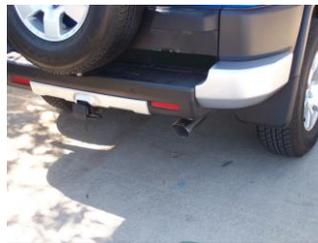
**6.** Install stainless steel tip #E. Clamp down. When you have everything in place, firmly tighten all bolts and clamps down securely. Use stainless steel cleaner and a Scotch Brite pad weekly to prevent tip from discoloration.
