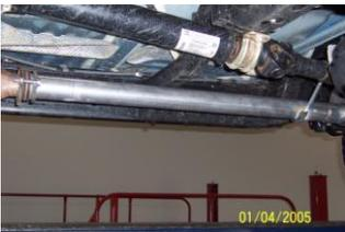
INSTALL HEAD PIPE #A ON TO YOUR EXISTING STOCK 2-BOLT FLANGE AND SECURE WITH BOLT KIT #F. INSERT WELDED HANGER INTO RUBBER GROMMET. DO NOT TIGHTEN
