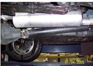
INSTALL MUFFLER #B ONTO HEAD PIPE 1-1/2" TO 2" WITH THE LOUVERS FACING TOWARDS THE CONVERTER. THE MUFFLER OUTLET SHOULD BE POSITIONED AT 12:00. USE A JACK STAND TO SUPPORT THE MUFFLER. USE CLAMP #E TO SECURE THE MUFFLER TO THE HEAD PIPE. DO NOT TIGHTEN. MUFFLER INLET IS LOOKING INTO THE LOUVERS.
