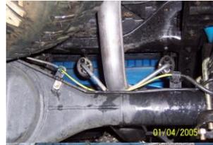
INSTALL THE OVERAXLE TAILPIPE #C INTO THE MUFFLER 1-1/2" TO 2". SECURE TO THE MUFFLER USING CLAMP #E. DO NOT TIGHTEN.
