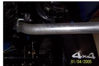
INSERT WELDED HANGERS INTO RUBBER GROMMETS.
