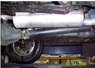
INSTALL MUFFLER #B ONTO HEAD PIPE 1-1/2" TO 2" WITH THE LOUVERS FACING TOWARDS THE CONVERTER. MUFFLER OUTLET SHOULD BE POSITIONED AT 12:00. USE A JACK STAND TO SUPPORT THE MUFFLER. USE CLAMP #E TO SECURE THE MUFFLER TO THE HEAD PIPE. DO NOT TIGHTEN. MUFFLER INLET IS LOOKING INTO THE LOUVERS.
