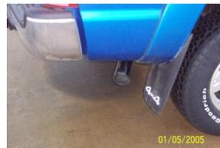
NEXT INSTALL YOUR STAINLESS STEEL TIP TO YOUR DESIRED LOOK. USE ANY ALUMINUM OR STAINLESS STEEL CLEANER TO POLISH YOUR TIP. MAKE SURE YOU HAVE A MINIMUM OF A 1" CLEARANCE ON ALL PIPES FROM ALL RUBBER BRAKE LINES, TIRES, SHOCKS, FUEL LINES, ETC. THEN TIGHTEN ALL CLAMPS AND HANGERS
