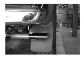
INSTALL THE STAINLESS TIP. USE A STAINLESS OR ALUMINUM CLEANER TO POLISH TIP. NOW TIGHTEN ALL HANGERS AND CLAMPS.
