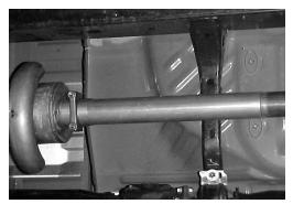
CUT STOCK EXHAUST 17-1/2" IN FRONT OF THE STOCK MUFFLER SLIDE THE HEADPIPE ONTO THE STOCK HEADPIPE USING CLAMP # E. THEN INSTALL THE MUFFLER ON HEADPIPE #A NO LESS THAN 1-1/2" TO 2" USING CLAMP #E. THE MUFFLER OUTLET WILL BE CLOCKED AT 12 O'CLOCK POSITION. INLET OF MUFFLER HAS LOUVERS FACING THE MOTOR.
