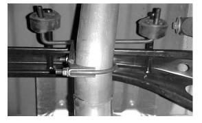
INSTALL REAR MUFFLER OE HANGER #F TO SUPPORT THE TAILPIPE.THE BOLTS FROM THE OE HANGER WILL BE FACING THE DRIVERSIDE. THIS HANGER ATTACHES TO THE TAILPIPE, NOT THE MUFFLER. DO NOT TIGHTEN.
