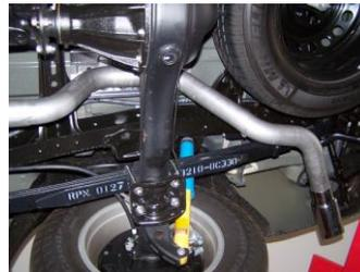
6. Install the overaxle tailpipe #E to the rear extension pipe #D. Use clamp #H to secure pipe. Do not tighten. Install hanger into rubber grommet.
