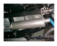
NEXT, SLIP THE MUFFLER #B ONTO THE HEADPIPE NO MORE THAN 2" AND NO LESS THAN 1  $\frac{1}{2}$ ". ATTACH TO HEADPIPE WITH CLAMP #G.
