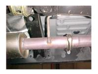
REMOVE STOCK EXHAUST BY UN-CLAMPING THE STOCK CLAMP AT THE HEADPIPE. BE CAREFUL NOT TO DAMAGE THIS CLAMP BECAUSE YOU NEED TO RE-USE IT. ONCE IT IS UN-CLAMPED, YOU WILL BE ABLE TO PULL THE STOCK **EXHAUST OFF THE** VEHICLE. MAKE SURE ALL FACTORY RUBBER GROMMETS ARE STILL IN FACTORY LOCATION, USE WD-40 TO AID YOU IN REMOVAL OF THE HANGERS FROM THE GROMMETS.
