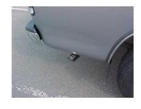
NOW INSTALL THE STAINLESS STEEL TIP USE ANY ALUMINUM OR STAINLESS STEEL CLEANER TO POLISH YOUR TIP. TIGHTEN ALL CLAMPS AND HANGERS STARTING FROM THE HEADPIPE BACK
