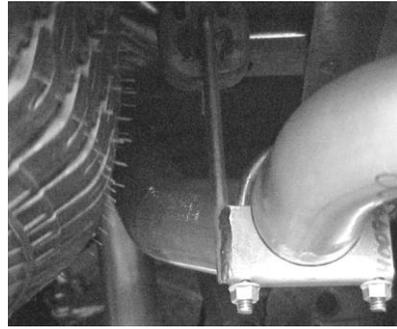
**SLIP OVERAXLE PIPE #C INTO THE OUTLET OF THE MUFFLER NO MORE THEN 2" AND NO LESS THEN 1 1/2". USE HANGER #G TO HANG THE OVERAXLE PIPE. THE SPARE TIRE MAY NEED TO BE LOSENED AND PUSHED TO THE REAR OF THE TRUCK TO GAIN CLEARANCE FOR INSTALLATION OF OVERAXLE PIPE. INSTALL THE EXIT PIPE #D AND CLAMP TO HANGER #G.**
