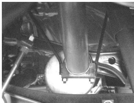
**NEXT, SLIP THE MUFFLER #B ONTO THE HEADPIPE NO MORE THAN 2" AND NO LESS THAN 1 1/2". ATTACH TO HEADPIPE WITH CLAMP #H. THEN USE HANGER #F TO HANG THE MUFFLER. THE MUFFLER OUTLET SHOULD BE AT 2 O'CLOCK. THE VERTICAL RODS ON THE HANGER WILL BE FACING TOWARDS THE FRONT OF THE VEHICLE AND INSERT HANGER INTO RUBBER GROMMET. MUFFLER INLET IS LOOKING INTO LOUVERS.**
