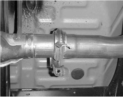
**REMOVE STOCK EXHAUST BY UN-CLAMPING THE STOCK CLAMP AT THE HEADPIPE. BE CAREFUL NOT TO DAMAGE THIS CLAMP BECAUSE YOU NEED TO RE-USE IT. ONCE IT IS UN-CLAMPED, YOU WILL BE ABLE TO PULL THE STOCK EXHAUST OFF THE VEHICLE. MAKE SURE ALL FACTORY RUBBER GROMMETS ARE STILL IN FACTORY LOCATION. USE WD-40 TO AID YOU IN REMOVAL OF THE HANGERS FROM THE GROMMETS.**
