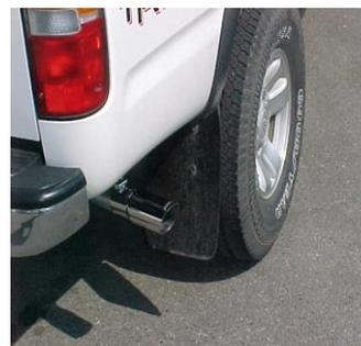
INSTALL THE STAINLESS TIP. USE A STAINLESS STEEL OR ALUMINUM CLEANER AND ANY SCOTCH BRITE PAD TO CLEAN. NOW TIGHTEN ALL HANGERS AND CLAMPS.
