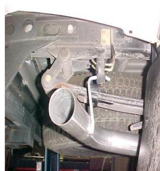
INSTALL WELDED HANGER INTO GROMMET.
