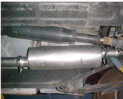
THEN INSTALL THE MUFFLER ON HEADPIPE #A NO LESS THAN 1-1/2" TO 2" USING CLAMP #E. THE MUFFLER OUTLET WILL BE CLOCKED AT 12 O'CLOCK POSITION. INLET OF MUFFLER HAS LOUVERS FACING THE MOTOR. DO NOT TIGHTEN.
