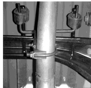
INSTALL REAR MUFFLER HANGER #C TO SUPPORT THE TAILPIPE. THE BOLTS FROM THE OE HANGER WILL BE FACING THE DRIVERSIDE. THIS HANGER ATTACHES TO THE TAILPIPE, NOT THE MUFFLER. DO NOT TIGHTEN.
