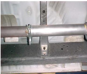
SLIDE THE HEADPIPE ONTO THE STOCK HEADPIPE ATTACHING CLAMP # E.
