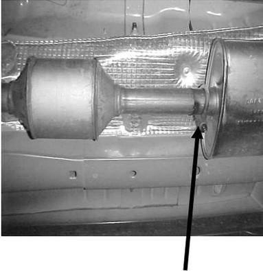
FOR EASIER REMOVAL OF THE FACTORY EXHAUST. CUT THE TAILPIPE BEHIND THE MUFFLER. THEN REMOVE THE FACTORY MUFFLER AT THE CLAMP IN FRONT OF THE MUFFLER. USE A JACK STAND TO SUPPORT THE CONVERTER ONCE EXHAUST IS REMOVED. **NOTE LEAVE ALL FACTORY RUBBER GROMMETS IN PLACE**
