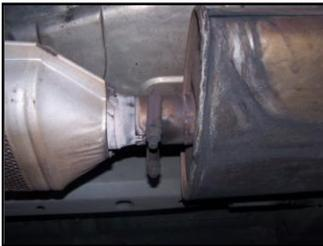
**2.** Unclamp and remove the stock exhaust from behind the catalytic converter. Use jack stand to support the converter. For easier removal and installation unbolt the rear hanger bracket.
