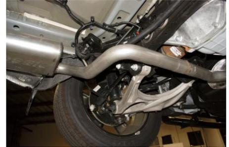
4. Install the driver side muffler assembly onto the factory pipe and into the factory rubber grommets. Do not tighten.
