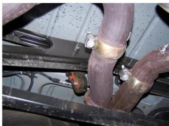
2. To remove the stock exhaust, unbolt the tailpipes at the clamps behind the over axle pipe. Then disengage hangers from the rubber grommets, and remove the rear tailpipes and mufflers. Now remove all other hangers from rubber grommets and unbolt the rest of the exhaust system at the 2 flanges in front of the stock muffler.
