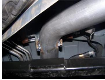
Install extension pipe #C into the muffler 1 1/2-2". Insert welded hanger into rubber grommet. Secure the muffler using clamp #E. DO NOT TIGHTEN.
