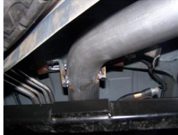
Install extension pipe #C into the muffler 1 1/2-2". Insert welded hanger into rubber grommet. Secure the muffler using clamp #E. DO NOT TIGHTEN.
