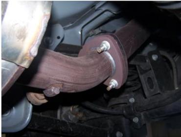
Lay out the exhaust on the floor so it looks like the drawing and compare parts with manual. Remove the stock exhaust from the 3 bolt flange just behind the muffler, then remove the back section, then the remaining stock exhaust from the 2 bolt flange in front of the muffler. Leave all rubber grommets in place. Use WD-40 to aid in removal of hangers.
