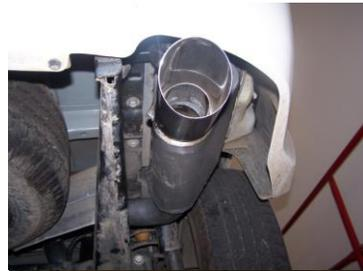
Install the over axle tail pipe w/welded resonator onto extension pipe, insert welded hangers into grommets and use clamp #E to secure pipes together. DO NOT TIGHTEN.
