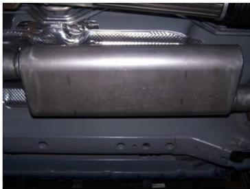
Install muffler #B onto head pipe #A 1 1/2-2" with the louvers facing towards the converter. Use a jack stand to support the muffler. Use clamp #E to secure the muffler to the head pipe. DO NOT TIGHTEN. Muffler inlet is looking into the louvers.
