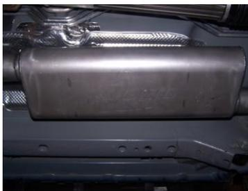
Install muffler #B onto head pipe #A 1 1/2-2" with the louvers facing towards the converter. Use a jack stand to support the muffler. Use clamp #E to secure the muffler to the head pipe. DO NOT TIGHTEN. Muffler inlet is looking into the louvers.
