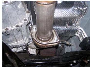
Install head pipe # A onto your existing stock flange and secure with bolt kit #F. DO NOT TIGHTEN.
