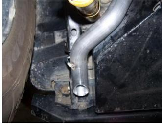
7. Adjust tailpipe to best fit your vehicle. Tighten all clamps working your way from the front to the back.
