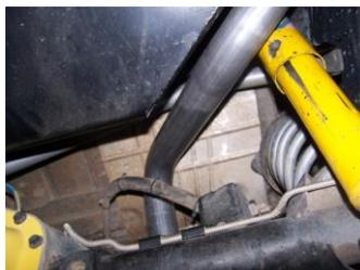
6. Install the over axle tailpipe #C into the muffler 1.5-2". Use clamp #E to secure tailpipe to muffler. Insert welded hangers into rubber grommets.
