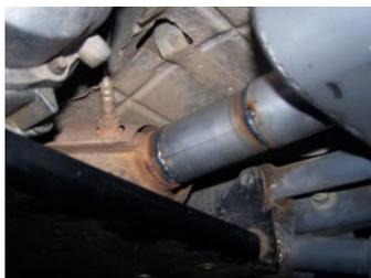
3. Install headpipe #A onto your existing stock pipe. This pipe will have to be welded to the converter. See picture.
