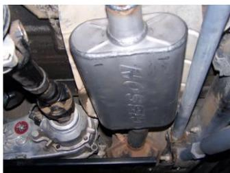
4. Install muffler #B onto headpipe #A 1.5-2" with the louvers facing towards the converter. Use a jack stand to support the muffler. Use clamp #D to secure the muffler to the headpipe. Do not tighten. Muffler inlet is looking into the louvers.
