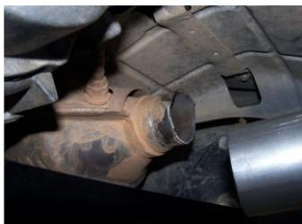
2. To remove the stock exhaust, cut it off at the converter. See picture. Disengage the welded hangers from the OEM rubber grommets. Use WD-40 to aid in this process. Do not damage or remove the rubber grommets as you will reuse them to mount your new system.
