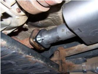
2. To remove the stock exhaust, unbolt the 2-bolt flange located in front of the muffler. Disengage the welded hangers from the OEM rubber grommets. Use WD-40 to aid in this process. Do not damage or remove the rubber grommets as you will reuse them to mount your new system. Now cut off tailpipe and remove exhaust.
