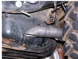
7. Adjust tailpipe to best fit your vehicle. Tighten all clamps and flanges working your way from the front to the back.
