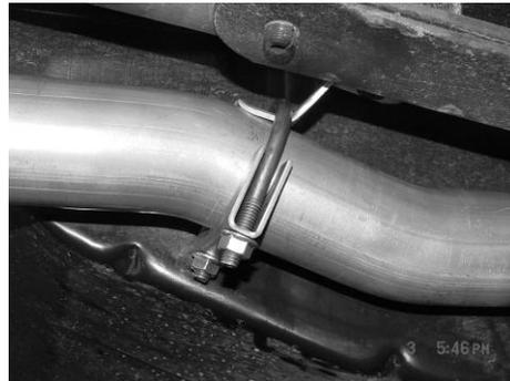
**5.) USE CLAMP #G ON TAILPIPE AND CONNECT TO THE FACTORY HANGER. DO NOT TIGHTEN.**
