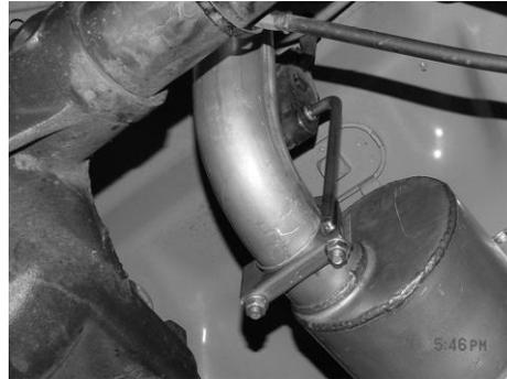
**4.) INSTALL TAILPIPE #C INTO MUFFLER AT LEAST 1-1/2" TO 2". INSERT O.E. HANGER #F INTO RUBBER GROMMET CLAMP TO ATTACH THE MUFFLER AND THE TAILPIPE. DO NOT TIGHTEN.**
