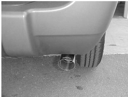
**6.) NEXT, INSTALL YOUR STAINLESS STEEL TIP TO YOUR DESIRED LOOK. TO CLEAN THE STAINLESS STEEL TIP USE A SCOTCH BRITE PAD AND ANY STAINLESS OR ALUMINUM CLEANER. YOU CAN NOW TIGHTEN ALL NUTS, BOLTS, AND CLAMPS STARTING FROM THE FRONT AND WORKING TO THE BACK.**
