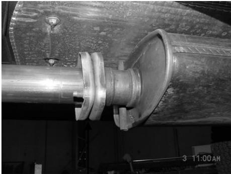
**1.) REMOVE STOCK EXHAUST BY UNCLAMPING AT THE FLANGE LOCATED JUST BEHIND THE CATALYTIC CONVERTER.**
