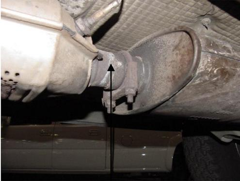
CUT 1" OFF BEHIND THE CONVERTER SO THE NOTCH IN THE MUFFLER WILL SLIP ON COMPLETELY.
