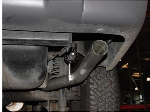
INSTALL OVERAXLE TAILPIPE #B INTO MUFFLER 1-1/2" TO 2". INSERT WELDED HANGER INTO RUBBER GROMMET, IF YOU REMOVED REAR HANGER BRACKET RE-INSTALL IT NOW. USE CLAMP #E TO SECURE TAILPIPE TO MUFFLER. DO NOT TIGHTEN.
