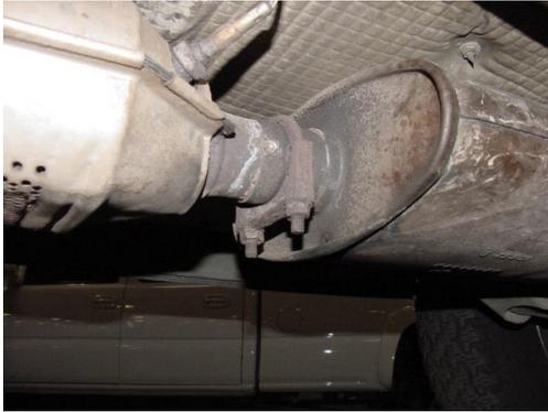
TO REMOVE STOCK EXHAUST UN-CLAMP IT FROM THE CLAMP LOCATED JUST BEHIND THE CATALYTIC CONVERTER. YOU MAY NEED TO HEAT THE CLAMP UP FOR EASIER REMOVAL. ALSO YOU MAY NEED TO UN-BOLT THE REAR TAILPIPE HANGER TO MAKE IT EASIER TO REMOVE STOCK EXHAUST AND INSTALL NEW EXHAUST.
