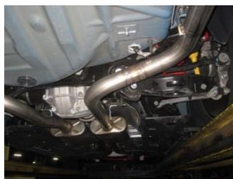
6. Install passenger side tailpipe/dual tip assembly #C. Insert all welded hangers into rubber grommets. Secure tailpipe with clamp #D. Do not tighten. Now go back and make sure the first two mufflers in the middle are level.
