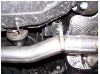
**MAKE SURE YOU HAVE A 1" CLEARANCE FROM ALL BRAKE LINES, SHOCK BOOTS, TIRES, FUEL LINES, ETC...**
