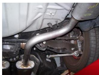
6. Install passenger side tailpipe/muffler assembly #C. Insert all welded hangers into rubber grommets. Secure tailpipe with clamp #D. Do not tighten.
