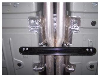
7. Now go back and make sure the first two mufflers in the middle are level. Then push up on factory cross member before tightening clamps. Then tighten X pipe. Next, with both tailpipes in place tighten all bolts and clamps securely.
