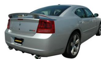
8. Use stainless steel cleaner and a Scotch Brite pad weekly to prevent tip from discoloration. Inspect all fasteners after 25-50 miles of operation and re-tighten as necessary.
