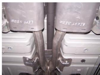
3. Install X pipe assembly #A assembly on to your front factory pipes and secure with factory clamps. Re-install factory cross member. Use a jack stand to support mufflers. Do not tighten.
