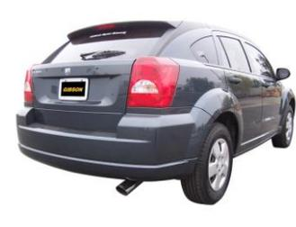
7. Install stainless steel tip. Clamp down. When you have everything in place, firmly tighten all bolts and clamps down securely. Use stainless steel cleaner and a Scotch Brite pad weekly to prevent tip from discoloration. Inspect all fasteners after 25-50 miles of operation and re-tighten as necessary.
