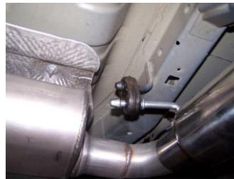
6. Next, slide exit pipe #D into muffler 1.5-2". Insert welded hanger into rubber grommet. Secure with clamp #F, do not tighten.
