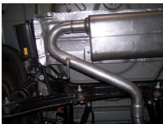
4. Next, slide inlet pipe #B onto headpipe #A. Insert welded hanger into rubber grommet. Secure with clamp #F, do not tighten.
