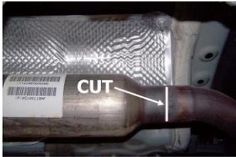
2. To remove the stock exhaust, cut right before the weld just after the stock resonator. Disengage the welded hangers from the OEM rubber grommets. Use WD-40 to aid in this process. Do not damage or remove the rubber grommets as you will reuse them to mount your new system.
