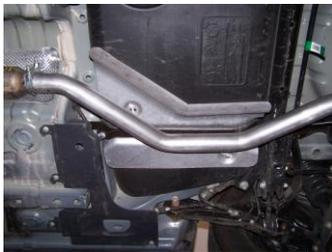
3. Slide headpipe #A onto stock resonator and secure with clamp #F. Use a jack stand to support the converter. Do not tighten clamp.
