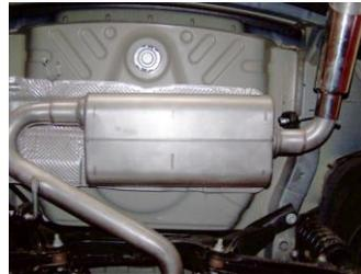
5. Now slide muffler #C onto inlet pipe 1.5-2". Secure with clamp #F, do not tighten.
