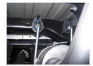
5. Slide band clamp #F onto muffler #B and attach with bolt kit #G. Do not tighten. Insert hangers into rubber grommets.
