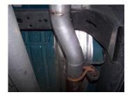
3. Install headpipe #A onto your existing stock headpipe and secure with clamp #E. Use a jack stand to support the converter.
