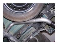
6. Install the over axle tailpipe #C into the muffler 1.5-2". Use clamp #E to secure tailpipe to muffler. Do not tighten. Insert welded hanger into rubber grommet.
