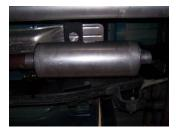
**3.** Install muffler onto head pipe #A 1½"-2" with the louvers facing towards the converter. Use a jack stand to support the muffler. Use clamp #E to secure the muffler to the headpipe. Do not tighten. Muffler inlet is looking into the louvers.
