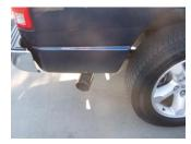
**6.** Install stainless steel tip #D. Clamp down. When you have everything in place, firmly tighten all bolts and clamps down securely. Use stainless steel cleaner and a Scotch Brite pad weekly to prevent tip from discoloration.
