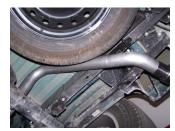
**5.** Install the overaxle tailpipe #C into the muffler 1½"-2". Use clamp #E to secure tailpipe to muffler. DO NOT TIGHTEN. Insert welded hanger into rubber grommet.
