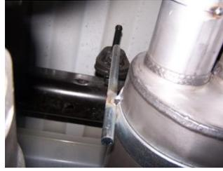
**4.** Slide band clamp #F onto muffler #B. Insert hangers into rubber grommet and attach with bolt kit #G. DO NOT TIGHTEN
