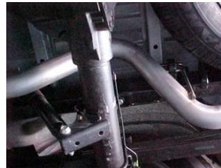
**5.** Install the overaxle tailpipe #C into the muffler 1 1/2"-2". Insert welded hanger into rubber grommet. Use clamp #E to secure tailpipe to muffler. DO NOT TIGHTEN.
