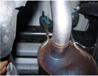
**1.** To remove the stock exhaust un-clamp it just behind the stock muffler. Then un-clamp stock muffler and remove. Leave all rubber grommets in place. Use WD-40 to aid in removal of exhaust.
