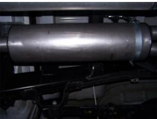
**3.** Install muffler #B onto head pipe #A 1 1/2"-2" with the louvers facing towards the converter. Use a jack stand to support the muffler. Use clamp #E to secure the muffler to the head pipe. DO NOT TIGHTEN. Muffler inlet is looking into the louvers.
