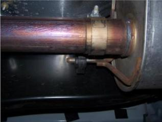
**2.** Install head pipe #A onto your existing stock front pipe and attach with clamp #E. Use a jack stand to support the converter. Insert welded hanger into rubber grommet.
