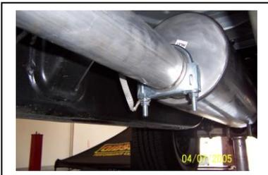
Install muffler # B onto head pipe # A 1-1/2" to 2" with the louvers facing towards the converter. Use a jack stand to support the muffler. Use clamp # F to secure the muffler to the head pipe. Do not tighten. Muffler inlet is looking into the louvers.
