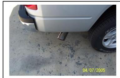
Install stainless steel tip. Clamp down. When you have everything in place, firmly tighten all bolts and clamps down securely. To clean stainless steel tip use any stainless steel cleaner.
