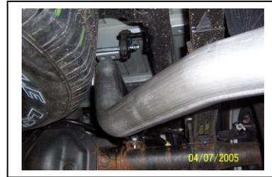
Install head pipe # A on to your existing stock front pipe and secure with clamp # E. Use a jack stand to support the converter. Insert welded hanger into rubber grommet. Do not tighten.
