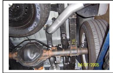
Install the over axle tailpipe # C into the muffler 1-1/2" to 2". Secure to the muffler using clamp # F. Do not tighten.
