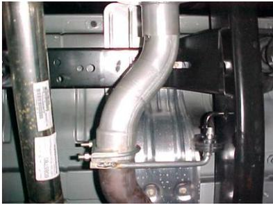
INSTALL HEADPIPE #A ONTO YOUR EXISTING STOCK FRONT PIPE AND SECURE WITH CLAMP #I. USE A JACKSTAND TO SUPPORT THE CONVERTER. INSERT WELDED HANGER INTO RUBBER GROMMET.
