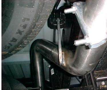
INSTALL THE OVERAXLE TAILPIPE #C INTO THE MUFFLER 1-1/2" TO 2". INSERT WELDED HANGER INTO RUBBER GROMMET. USE CLAMP #F TO SECURE TAILPIPE TO THE MUFFLER. DO NOT TIGHTEN.
