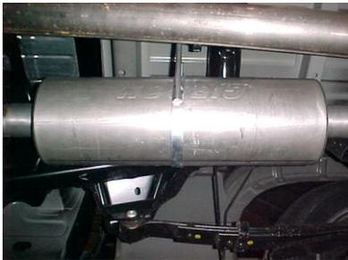
INSTALL MUFFLER #B ONTO HEADPIPE #A 1-1/2" TO 2" WITH THE LOUVERS FACING TOWARDS THE CONVERTER. USE A JACK STAND TO SUPPORT THE MUFFLER. USE CLAMP #F TO SECURE THE MUFFLER TO THE HEADPIPE. DO NOT TIGHTEN. MUFFLER INLET IS LOOKING INTO THE LOUVERS.
