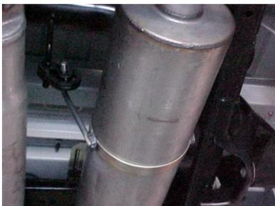
SLIDE BAND CLAMP #G ONTO MUFFLER #B. INSERT HANGERS INTO RUBBER GROMMETS.
