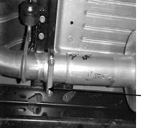
UN-CLAMP THE STOCK EXHAUST IN FRONT OF YOUR MUFFLER AND REMOVE. FOR AN EASIER REMOVAL OF THE EXHAUST CUT THE TAIL PIPE BEHIND THE STOCK MUFFLER. SLIDE HEADPIPE #A ON TO THE STOCK CONNECTOR PIPE. USE CLAMP #G TO ATTACH IT. DO NOT TIGHTEN. RAISE THE VEHICLE UP AND SUPPORT IT WITH A JACKSTAND. LEAVE ALL FACTORY RUBBER GROMMETS IN PLACE.
