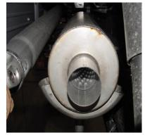
SLIDE MUFFLER WITH BAFFLES FACING FORWARD TOWARDS CONVERTER ONTO THE HEADPIPE NO LESS THEN 1<sup>1</sup>/<sub>2</sub>" AND NO MORE THAN 2". MUFFLER INLET IS LOOKING INTO LOUVERS.
