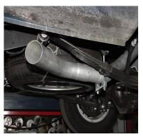
INSTALL EXIT PIPE #D USING CLAMP #H TO ATTACH TO THE OVER AXLE PIPE. DO NOT TIGHTEN. ROTATE PIPES UNTIL EVERYTHING IS LEVEL. ONCE YOU HAVE EVERY THING IN POSITION THEN TIGHTEN ALL CLAMPS AND HANGERS.
