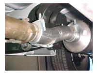
INSTALL HEADPIPE #A ONTO YOUR EXISTING STOCK FRONT PIPE AND SECURE WITH CLAMP #I. INSERT HANGER INTO RUBBER GROMMET.
