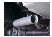
INSTALL EXIT PIPE #D OVERAXLE PIPE. ROLL TURNOUT PIPE UNTIL YOU HAVE IT AT THE CORRECT ANGLE FOR YOUR TRUCK AND CONNECT WITH CLAMP #F. BUT DO NOT TIGHTEN.
