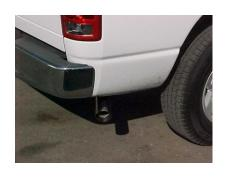
INSTALL STAINLESS STEEL TIP. WHEN YOU HAVE EVERYTHING IN PLACE, FIRMLY TIGHTEN ALL BOLTS AND CLAMP DOWN SECURELY. TO CLEAN STAINLESS STEEL TIP USE ANY STAINLESS STEEL CLEANER AND SCOTCH BRITE PAD.
