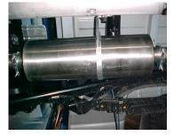
INSTALL MUFFLER #B ONTO HEADPIPE #A 1-1/2" TO 2" WITH THE LOUVERS FACING TOWARDS THE CONVERTER. USE A JACK STAND TO SUPPORT THE MUFFLER. USE CLAMP #F TO SECURE THE MUFFLER TO THE HEADPIPE. DO NOT TIGHTEN.
