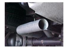
INSTALL EXIT PIPE #D OVERAXLE PIPE. ROLL TURNOUT PIPE UNTIL YOU HAVE IT AT THE CORRECT ANGLE FOR YOUR TRUCK AND CONNECT CLAMP. BUT DO NOT TIGHTEN.
