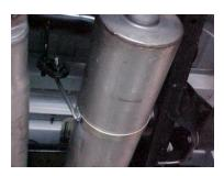
SLIDE BAND CLAMP #G ONTO MUFFLER #B. INSERT HANGERS INTO RUBBER GROMMETS. SUGGESTED TOOLS: 1/2" WRENCH, 9/16" SOCKET, 15MM SOCKET, HACKSAW, JACKSTAND,Wd-40
