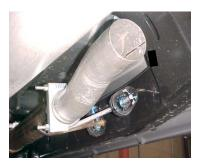
LAY OUT THE EXHAUST ON THE FLOOR SO IT LOOKS LIKE THE DRAWING AND COMPARE PARTS TO THE MANUAL. **TO REMOVE THE STOCK EXHAUST UN-CLAMP IT JUST IN FRONT OF THE MUFFLER.** YOU MAY NEED TO HEAT IT UP FOR EASIER REMOVAL. LEAVE ALL RUBBER GROMMETS IN PLACE.
