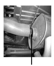
DO NOT REMOVE THE STOCK HEADPIPE.CUT 1 ½" IN FRONT OF STOCK MUFFLER.
